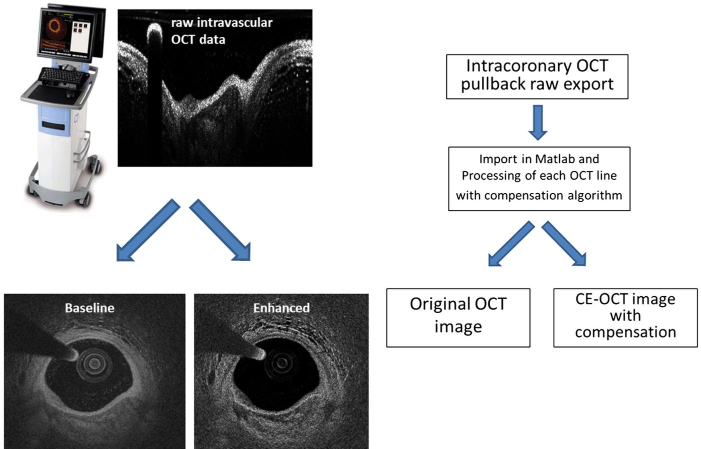
**Fig. 2.** Flow chart of data processing. Intravascular OCT raw data obtained from the OCT scanner were imported in Matlab and processed with attenuation compensation along each OCT A-Scan. Contrast enhanced results after compensation were plotted in polar representation against baseline OCT plot without compensation.
