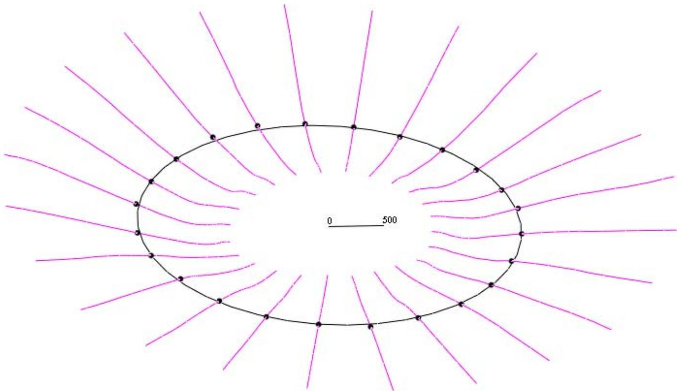
**FIGURE 4.** The scleral reference structure: anterior sclera (magenta), scleral representatives located at 1700 to 1800  $\mu\text{m}$  from the axis of the BMO cylinder (black dots), and scleral ellipse (black ellipse, which lies in the scleral plane).  $LD_{AS}$  is the distance from this plane to the lamina. A 500- $\mu\text{m}$  measure is included to illustrate scale.
